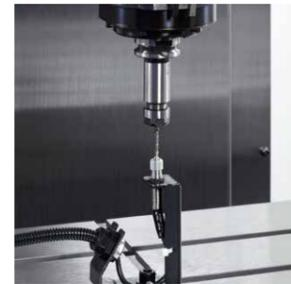
**Tool breakage detector, touch type**
