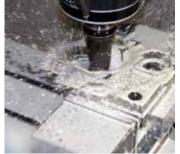
Large hole drilling using high-torque specs
