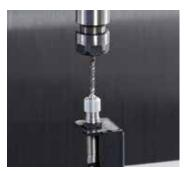
Tool breakage detector (touch type)
