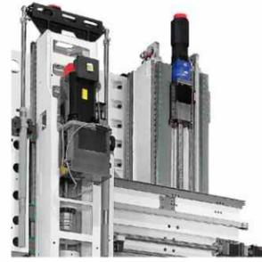
W-axis features twin ball screws and twin servo motors.
