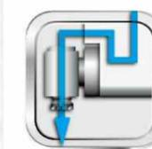
**Angular head center coolant mechanism (UAC)**
