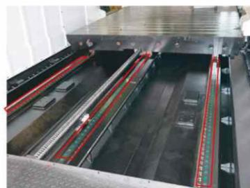
X-axis three linear guideways design MW-X43
