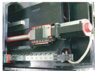
MW three-axis direct-connected drive advantage
