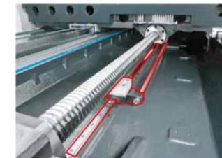
X-axis screw support mechanism
