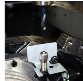
**Tool breakage detector, touch type**
