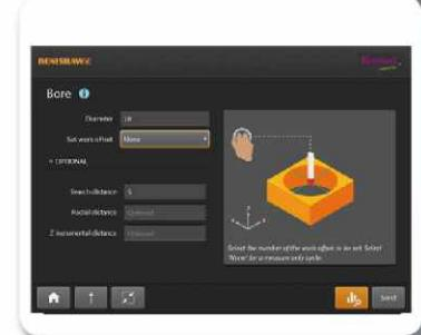
Graphical user interfaces for part setting, inspection, tool setting
