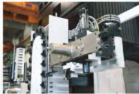
1.The vertical and horizontal tool magazine
