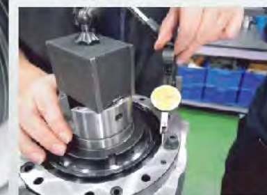
• End surface flatness correction
