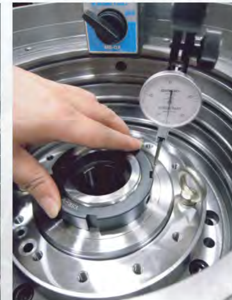
• Adjust teeth clearance
