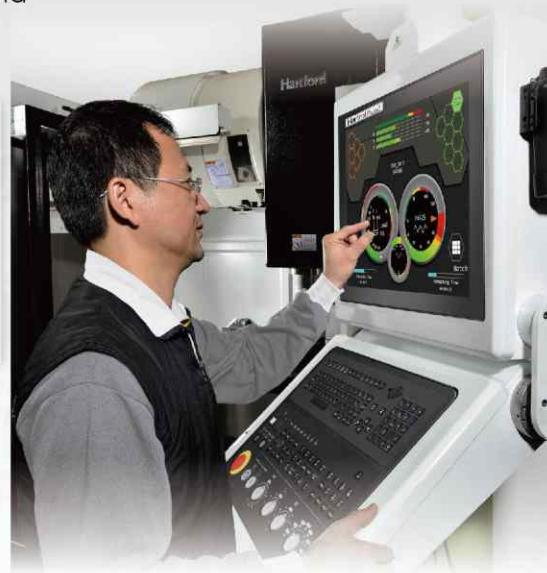
The main technologies of Hartford smartcenter include intelligent managing system, status monitoring, alarm predicting, machine status diagnosis, crash preventing, 3D program simulation, machining efficiency improving...etc. All the intelligent functions help you control the machine status and assure the job quality.
