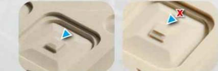
Tool center point in 5-axis (X,Y,Z,B,C) positions accurately.
