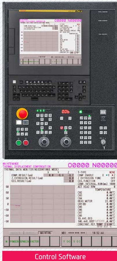
Structure thermal displacement error correction
