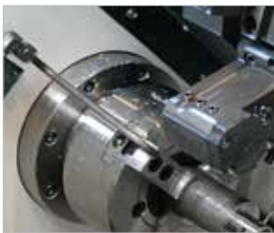
Chuck Air Blow (Upper Chuck)
