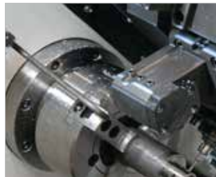
Chuck Air Blow (Upper Chuck)
