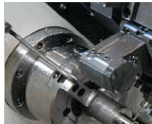
Chuck Air Blow (Upper Chuck)
