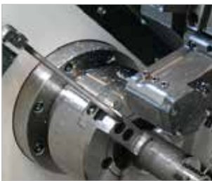
Chuck Air Blow (Upper Chuck)
