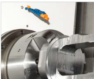
Chuck Coolant (Upper Chuck)
