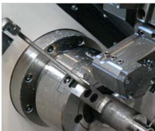
Chuck Air Blow (Upper Chuck)
