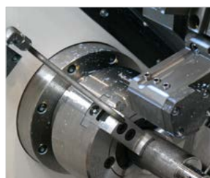
Chuck Air Blow (Upper Chuck)
