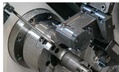
Chuck Air Blow (Upper Chuck)
