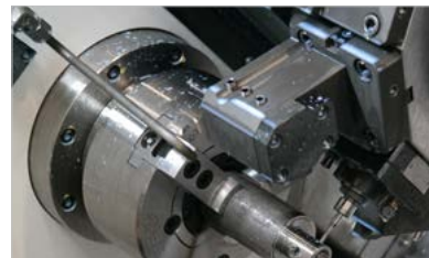
Chuck Air Blow (Upper Chuck)
