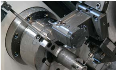
Chuck Air Blow (Upper Chuck)
