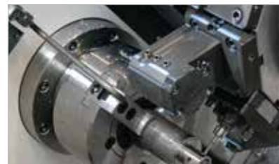
Chuck Air Blow (Upper Chuck)
