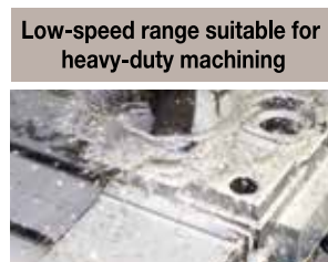
Low-speed range suitable for heavy-duty machining Large hole drilling using high-torque specs Machining details Hole diameter: D40 mm Material: Carbon steel
