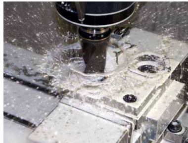
Large hole drilling using high-torque specs
