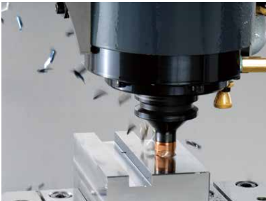
Grooving using standard specs
